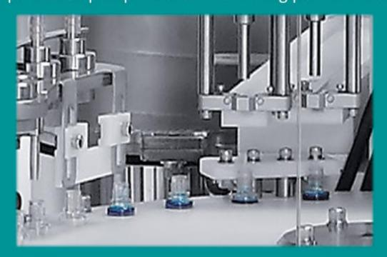
Easy and quick adjustment for Nib and Cap mechanism for absolute reliable accuracy
